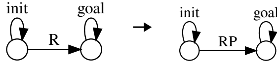
Figure 7: Second rule - Going from the start point to the goal without crossing other nodes is inherently safe and marked as "Reachable Preferred".
