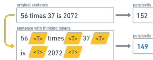
Figure 1: Illustration of 'thinking tokens' (marked as <T>) in a sentence which requires a complex calculation and the positive impact of this approach on perplexity of the model (lower is better).
